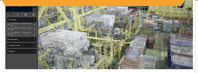
The Airscope team did an extensive two-part capture of up to 1548 hours of work. They initiated the process with laser scanners and drones capturing 6947 laser scans and 16680 drone images for a highly detailed and accurate capture of the platform.
